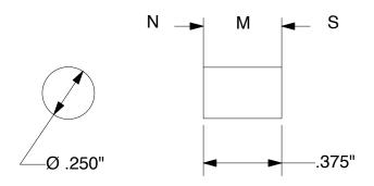
MATERIAL: 0.250" DIA X .375" THK NEO 42 NICKEL PLATED & MAGNETIZED
